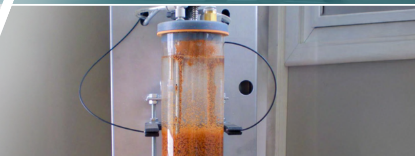
04 Automatic flocculation controller
